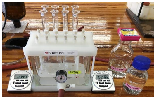
Figure 6. Vacuum manifold with attached cartridges
