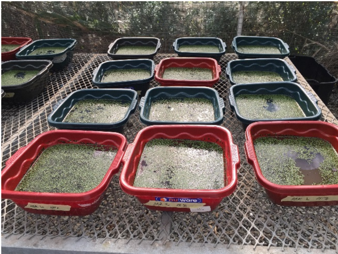
Figure 1. Dilution Row of ABR 7 (first 3 containers contain 100% WW and so on).
