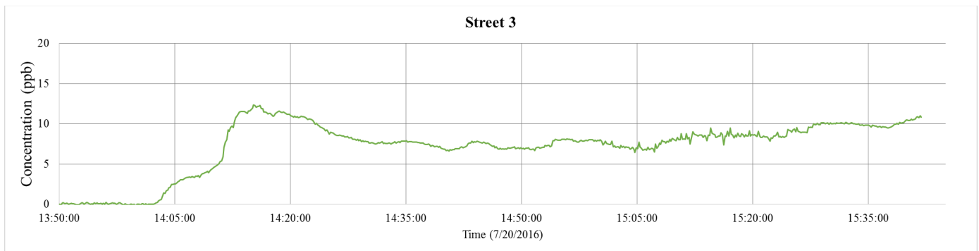
Figure 13. Street 3 Fluorescein Tracer Test (I)
