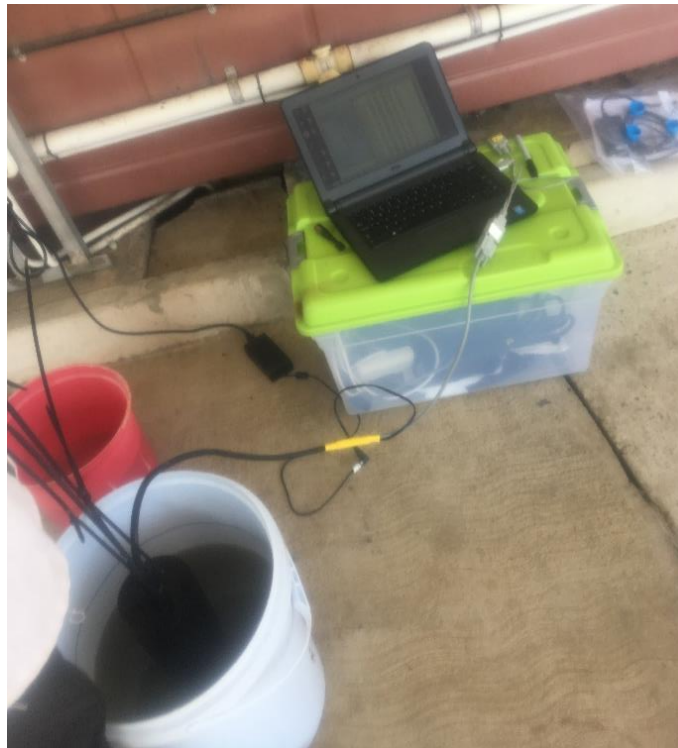
Figure A3: Fluorometer held by zip ties while connected and collecting real-time data
