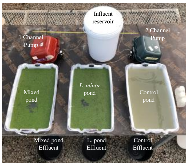
Figure 4: Continuous flow setup with Mixed, L. minor , and Control ponds fed by influent reservoir.
