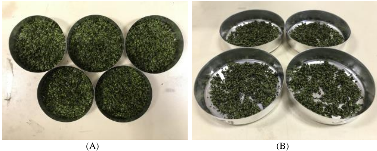
Figure 7: 5 g dewatered duckweed in metal weighing trays before drying (A) and after one day of drying (B).
